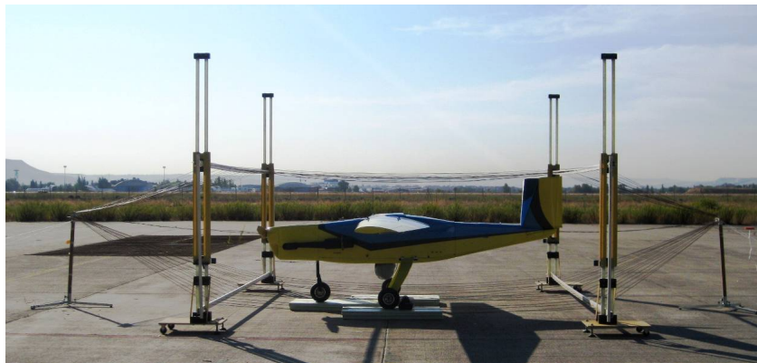
Figure 5.7: DCI test setup using coaxial return of SIVA-UAV in INTA's Open Area Test Site (OATS).
