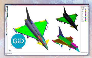
Generate meshes which preserve all ohmic connectivities and take into account electromagnetic phenomena. One of the fastests meshers in the world, the power of billions of cells within seconds.
